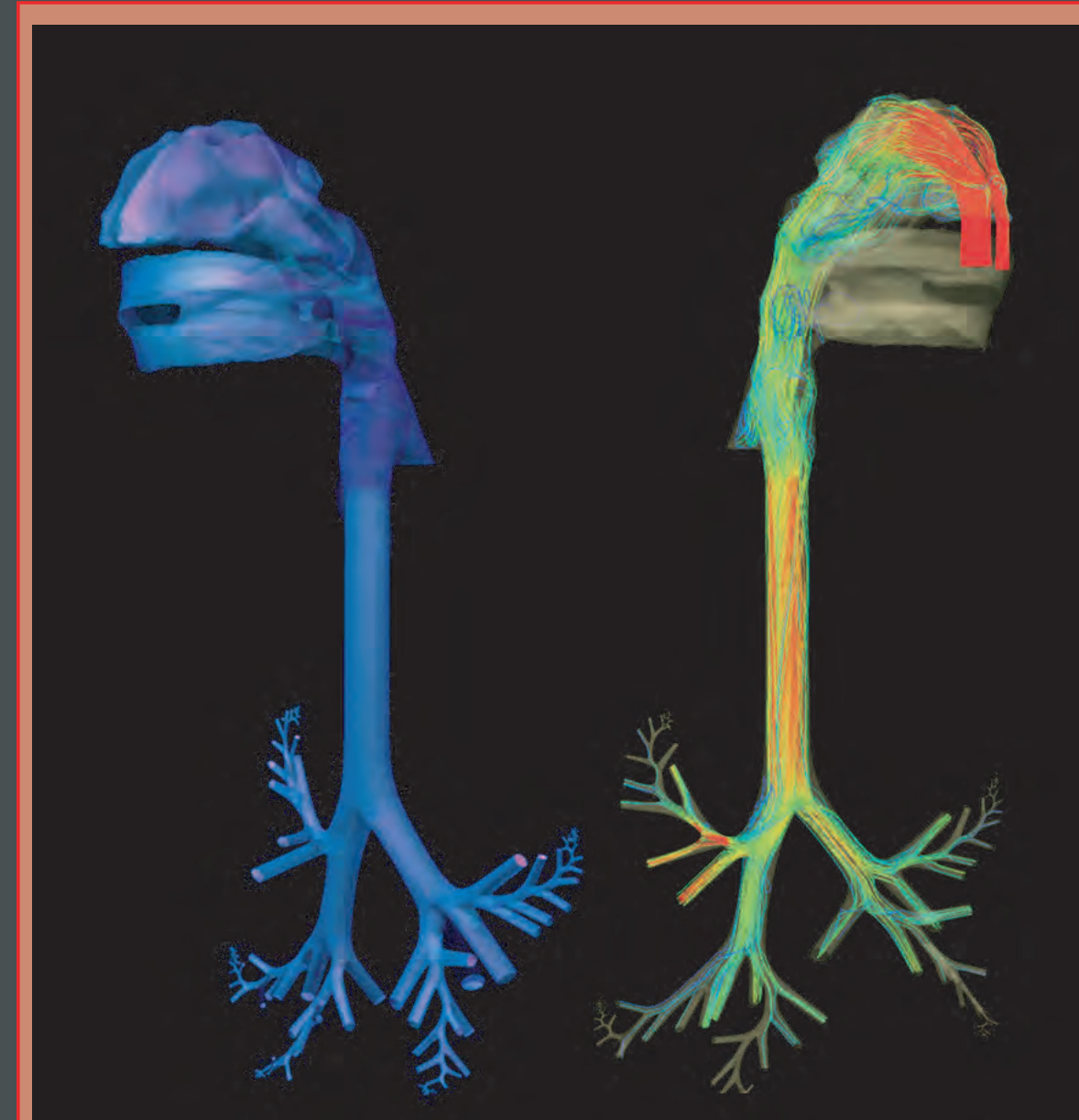
Figure 5 The internal structures were combined to create a three-dimensional morphologically realistic model of the human respiratory tract from the nares to the alveoli (left). To confirm the model was free from surface imperfections we prepared a computational mesh, a process which requires a watertight surface and performed a trial CFD run. Traces of velocity magnitude are shown for inhalation laminar flow (right).
